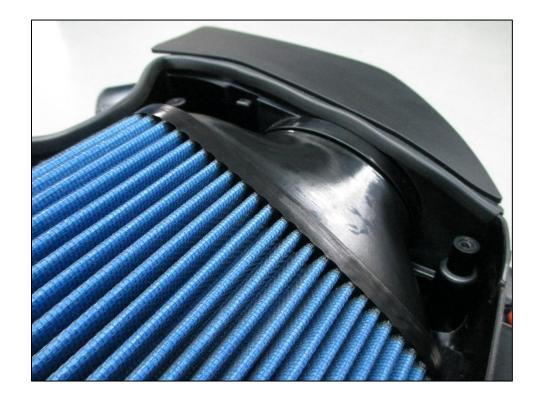
7. Install the supplied foam strip along the underside of the front edge of the carbon fiber Dinan airbox lid as shown. Trim the length of the foam strip to fit as needed.
