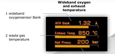
Specifies the current value of wideband oxygen sensor Bank 1; measures the residual oxygen content in the exhaust gas;  $\lambda > 1$  = lean mixture;  $\lambda < 1$  = oily mixture; Range is between 0.65 and 2.5
