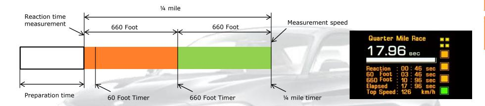
The quarter mile display of F2xDGA serves the riders to perform a drag racing with exact measurements. Due to a short preparation time of 10 seconds, the driver can prepare for the race. The traffic light in the right pane indicates the start time. In the light of the last green signal timing begins.
