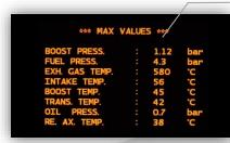
Specifies the maximum value of the current drive; When the switch off the ignition deletes these values
